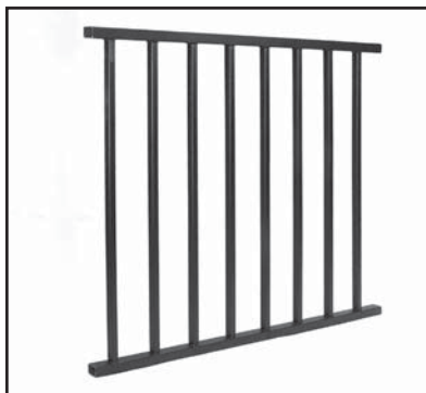
Top / bottom rail measure 1-1/4" x 1-1/4" 5/8" Square Infill
