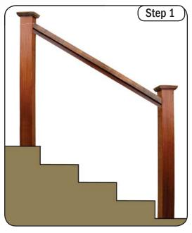
FrameWork Posts should be set in place. Top rail should be temporarily fastened into place, so the cable brace can be added later.
