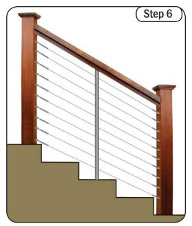
Finish Rail Once the cable brace is set and the framework is complete, run the cables and tension to complete the rail system.
