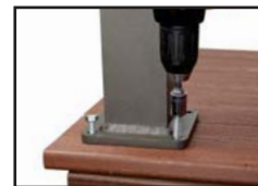
Fasten Post to Deck Surface
