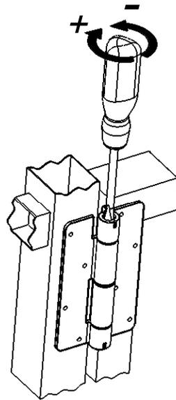
The hinge should be inspected annually, or more frequently if the gate is used often. Spring tension adjustments should be made as needed. The hinge should be regularly lubricated by spraying an oil based lubricant into the area of the cams and barrel.
