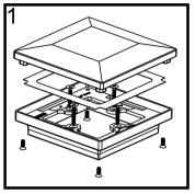
1. The following components are included with the FortressAccents 3.5", 4", 5", and 6" Flat Pyramid Caps: Post Cap, Post Cap Base, Light Slot Cover, 4 - Machine Screws, and 4 - #10 X 3/4" Wood Screws. Note: 5" and 6" Flat Pyramid Caps include a Composite Adapter with 4 -Pan Head Machine Screws.
