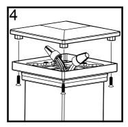
4. Before installing the post cap, make the connections on all of the LED cap modules you plan to use. Connect the field wiring to the transformer and turn on the lights to verify that the wiring is correct. Install the post cap cover with the provided fasteners.
