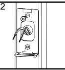
2. Metal Post Installations - Pre-drill screw holes using a 5/32" drill bit.
