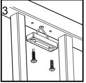
3. Metal Installations - When installing LED Universal Light on metal surfaces pre-drill screw holes using a 5/32" drill bit. Using a 3/8" drill bit drill a hole to allow for wires to be routed through the surface. Hole must be placed so that the LED Universal Light housing does not pinch wires. Route wires through hole. For some installations, railing must be disassembled to route wires through railing. Attach the LED Universal Light with supplied metal screws.
