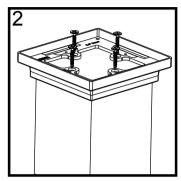
2. Place the Post Cap Base on the post and mark hole locations. Pre-drill holes with a 1/8" drill bit. Using the 4 supplied #10 X 3/4" Wood Screws, attach the Post Cap Base to post.
