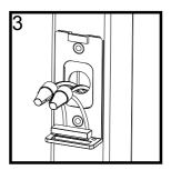
3. Strip the insulation back ½" from the 18-2 gauge wires and the LED Vertical Post Light feed wires. Using the supplied waterproof wire nuts connect wires. Wire connections can also be made below the deck surface. Note: Polarity must be maintained. Always connect the same side of 18-2 gauge wire with the same polarity (i.e. positive) marked on the LED Vertical Post Light wires. LED Vertical Post Light feed wires are 60" long.
