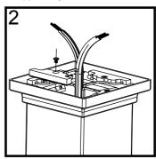
2. Place each LED module into an indention in the FortressAccents post cap base with the LED's facing down. Secure the LED module with provided screws. You may eliminate the light emitted from any side of the FortressAccents post cap by clipping the wire of the unneeded LED module and wrapping the ends of wire with electrical tape.
