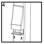
4. Carefully tuck wires out of the way. Place LED Vertical Post Light Cover over the installed LED Vertical Post Light Base and slide downward until cover is fully in place. Using the two supplied machine screws secure the cover to the base.
