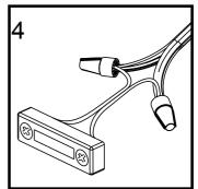
4. Strip the insulation back ½" from the 18-2 gauge wires and the LED Universal Light feed wires. Using the supplied waterproof wire nuts connect the wires. Note: Polarity must be maintained. Always connect the same side of 18-2 gauge wire with the same polarity (i.e. positive) marked on the LED Universal Light wires.
