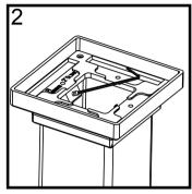
2. Place the Post Cap Base on the post. Using the supplied 2.5mm Allen Wrench tighten the two set screws. Adjust the screws to center and level the Post Cap on the post.
