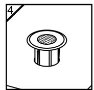
4. Feed wires through 1" hole. Insert LED Surface Mount Light into hole. Using a rubber mallet tap the light into the hole until the LED Surface Mount Light flange is flush with the deck surface.
