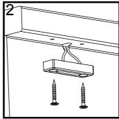
2. Wood and Composite Installations - When installing LED Universal Light on wood or composite surfaces pre-drill screw holes using a 1/16" drill bit. Using a 3/8" drill bit drill a hole to allow for wires to be routed through the surface. Hole must be placed so that the LED Universal Light housing does not pinch wires. Route wires through hole. Attach the LED Universal Light with supplied wood screws.
