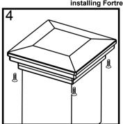
4. Secure Post Cap with the 4 Machine Screws that were removed in step 1.
