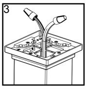
3. Strip the wire insulation back ½" from the field wiring. Connect wires with provided waterproof wire nuts. Wire connections can also be made below the deck surface. Note: Polarity must be maintained. Always connect the same side of 18-2 gauge wire with the same polarity (i.e. positive) marked on the LED Cap Light Kit.
