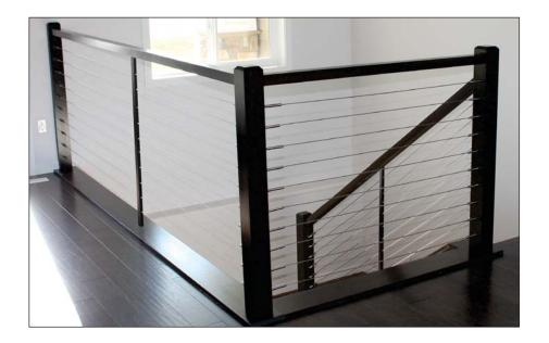
Cable braces are non-structural railing supports designed to help maintain spacing to avoid cable deflection over 4" to keep within code parameters. Designed for wood railing frames (with or without bottom rails) up to 42" high with 12 pre-drilled holes at a 3-1/8" on center spacing.
