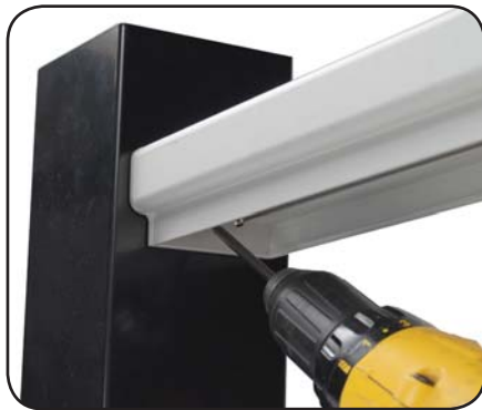
Series 200 Terminating into Post - 2 Use 2 ea. included screws to attach end plate to top rail. Then use holes that were created to connect top rail into post or column.
