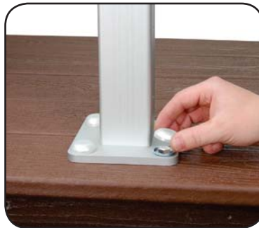
Step 5: Press bolt caps onto cup washer to finish post
